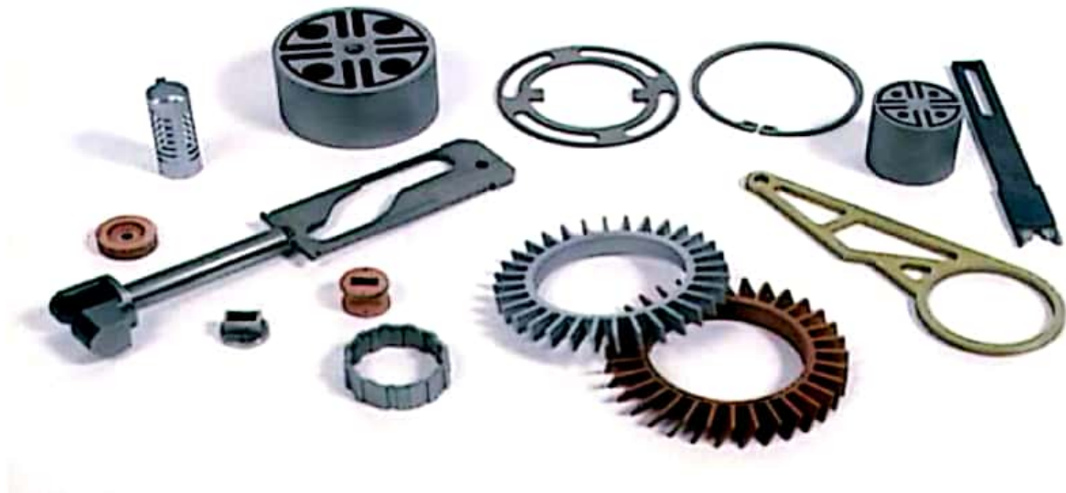
Figure 14: Difficult internal parts made by EDM process
