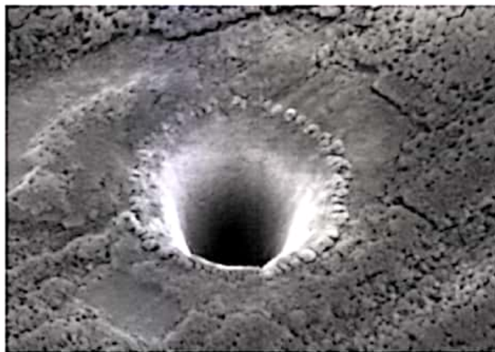
Figure 18: SEM micrograph hole drilled in 250 micro meter thick Silicon Nitride with 3 rd harmonic Nd: YAG laser
